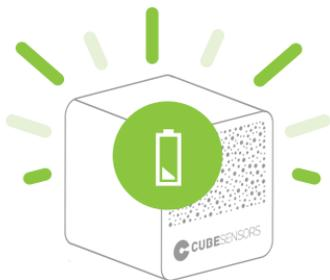
If a Cube **blinks green after the shake**, its battery is running low. It will still be collecting measurements for a few days, but you should connect it to a power source as soon as possible to recharge it and get the full experience.
